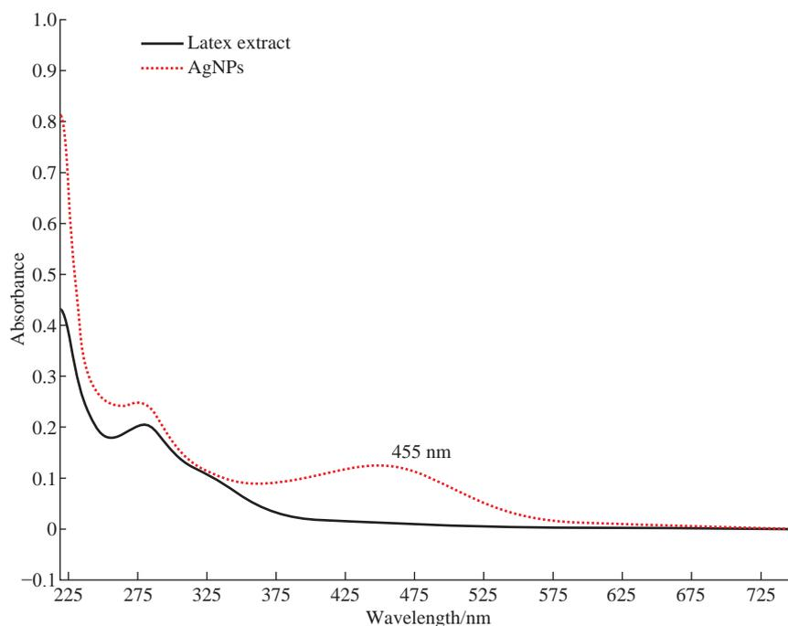
**Fig. 2** UV-visible spectra of  $\text{AgNO}_3$  particles with 3% latex.
