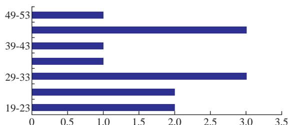
**Fig. 4** Particle size distribution histogram of silver NPs determined from TEM image. The minimum and maximum diameters of the particles were 19.83 nm and 52.88 nm.
