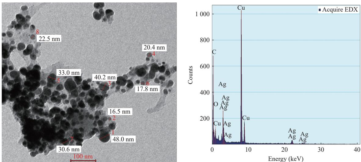
**Fig. 5** TEM with EDX micrograph (100nm and 50nm) of AgNPs synthesized by *Luisia tristis*
