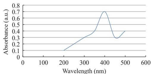
Fig. 2 UV–Vis spectroscopy analysis of AgNPs synthesized.
