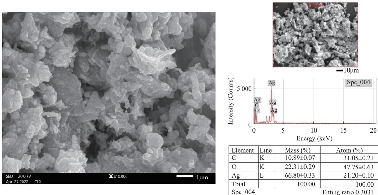
Fig. 4 SEM micrograph (100 and 50 nm) of AgNPs synthesized from *Luisia tristis*.
