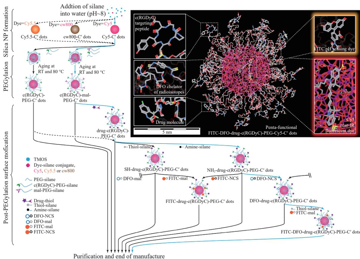
**Fig. 5** Scheme illustration of synthesis process of USNPs introduced with PEG for multiple surface modification by an insertion method [93]. © 2017 American Chemical Society.
