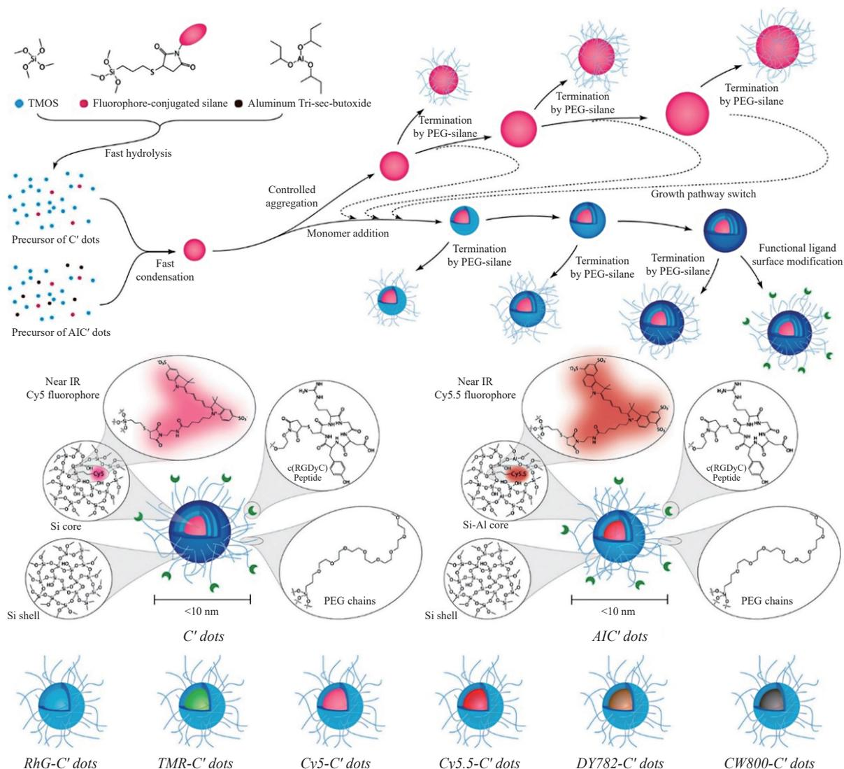
**Fig. 4** Scheme illustration of water-based fluorescent USNPs growth pathways, together with the chemical structures of produced particles [9]. © 2015 American Chemical Society.
