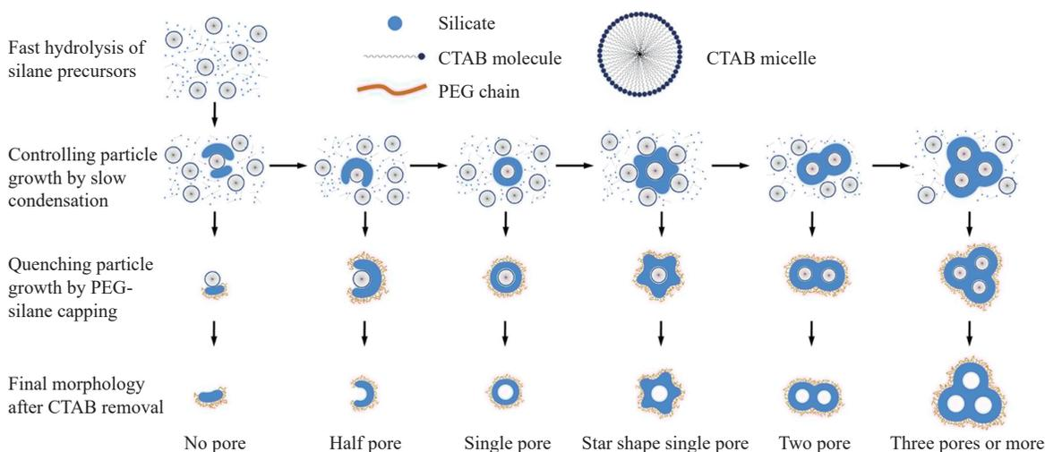
**Fig. 1** Diagram of how to synthesize USNPs with various particle sizes and shapes using the soft template method [36]. © 2013 American Chemical Society.
