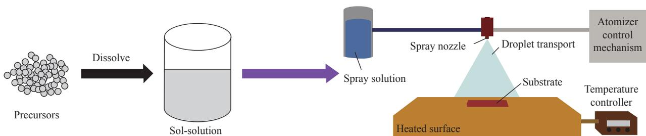
Fig. 1 Experimental preparation procedures of the monolayer and bilayer thin films
